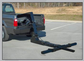
The Snatcher bolts into the bed of your pickup truck and is ideal for light-duty towing such as repossession work, moving vehicles around parking lots or moving vehicles in parking ramps or garages where height clearance may be an issue.
