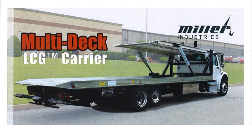
The combination of proven technology and reliability of a 16 Series Aluminum LCG™ (Low Center of Gravity) Carrier with an auxilary deck system. The Multi-Deck Carrier is available in deck lengths from 24-26 feet for hauling up to 3 vehicles as well as 30 foot decks for transporting up to 4 vehicles.
