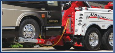
Century offers the Low Rider Underlift to provide the strength and durability you need for your toughest tows while still providing the lowest profile stinger. The Low Rider provides you with 144" of reach while the "Coach" Low Rider provides additional reach up to 160" to haul those difficult pumpers, packers, coaches, and fire trucks.
