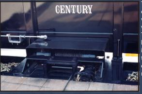
The 20 series carrier comes standard with a 12,000 lb. worm gear winch. The optional 12,000 lb. planetary winch is shown here with the optional winch cover and 4-way roller guide.
