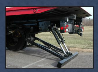
A hydraulic dock stabilizer is standard on all 30 series carriers, and is available in lieu of the wheel lift on the 20 series carrier. Century's mounting plate above the stabilizer accommodates for the optional pintle hook.
