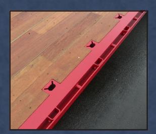
The optional outside stake pockets with rub rails and pipe spools can be combined with additional key slots to provide more versatile tie down options.
