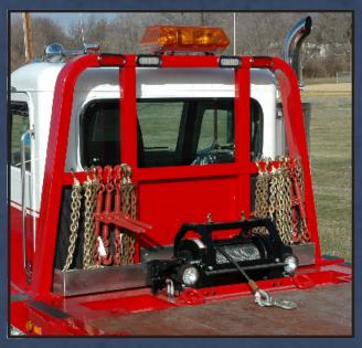
The steel tube cab protector (standard on the 30 series and optional on the 20 series) includes a rack for your chains and binders. Steel wire mesh can be added for additional protection of the rear window. A stainless steel chain tray is available for the stationary cab protector.
