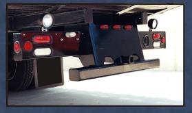
The 20 series carrier, show here, has a fixed stabilizer and the receiver for a trailer hitch. The standard tail-light housings are equipped with shock-mounted & sealed tail, back-up, and marker lights for
