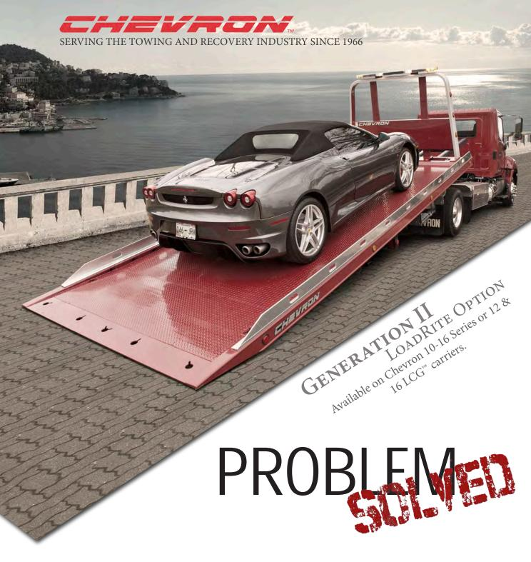
Exotic, High Performance or Low Clearance vehicles are no problem for Chevron's Generation II LoadRite carriers. The LoadRite features a unique "drop deck" design with a slopped tail section that improves the load angle an additional 3 degrees. For ease in securing your load, the LoadRite option on a steel carrier features bi-directional chain locks along the inside rail every 12 inches.
