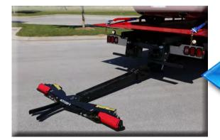
To provide quick and easy hook ups without the hassle of L Arms for towing a second vehicle, your LoadRite II can be equipped with the AutoGrip II wheel lift.
