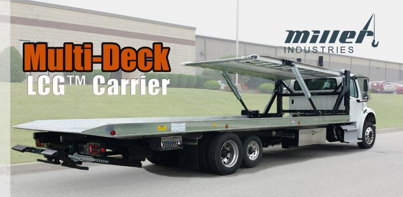
The combination of proven technology and reliability of a 16 Series Aluminum LCG<sup>™</sup> (Low Center of Gravity) Carrier with an auxilary deck system. The Multi-Deck Carrier is available in deck lengths from 24-26 feet for hauling up to 3 vehicles as well as 30 foot decks for transporting up to 4 vehicles.
