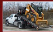
With a deployment of the deck taking approximately 60 seconds and the ability to drive equipment on and off rather then winching it up a deck, most companies report time savings of 30% to 40% over conventional carriers.
