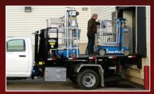
The optional loading dock feature allows the operator to raise the deck up to 8" so that equipment can be loaded or unloaded directly onto a loading dock.
