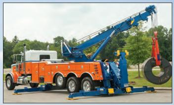
For maximum stability, the 1150R can be ordered with the dual "H" beam outrigger system and HHU underlift.
