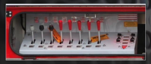
This option adds manual controls to the passenger side and replaces the panels as shown on the lower right of the previous slide.
