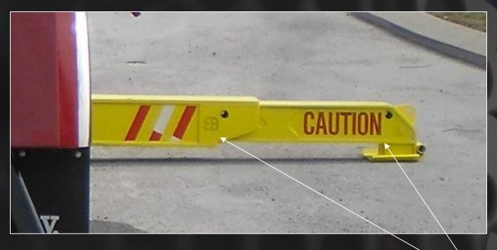
Note holes that allow legs to be pinned fully in or out during a side pull
