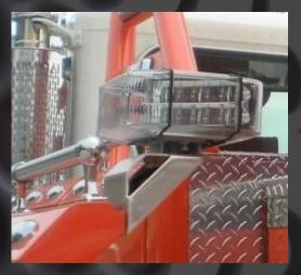
For Rotator top-beam front outrigger, use 124002812-includes bracket
