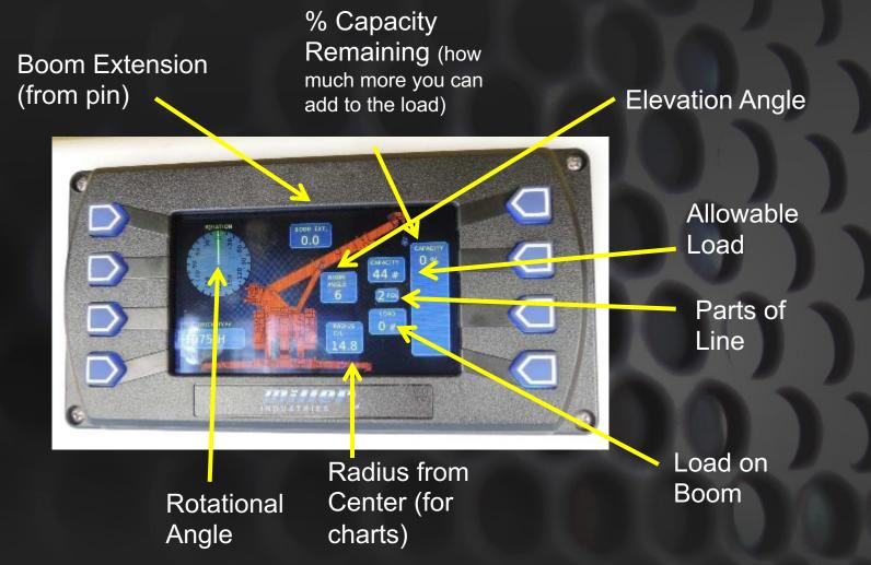
2 touch screens are standard with an MMO and MMGO system. But only the rear display shows load information with the optional MMGO system.
