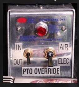
Left – Single Action – also shows the yellow knob for the pusher axle air pressure adjustment. Allows for manual PTO engagement if there is an electrical failure.
