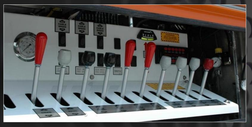
Allows for a maximum of 1 deck drag winch. Not available with two or more auxiliary winches. Includes manual control handles for all outriggers
