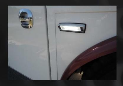
Also functions as marker light & flasher light when used with Flasher Control Power Unit
